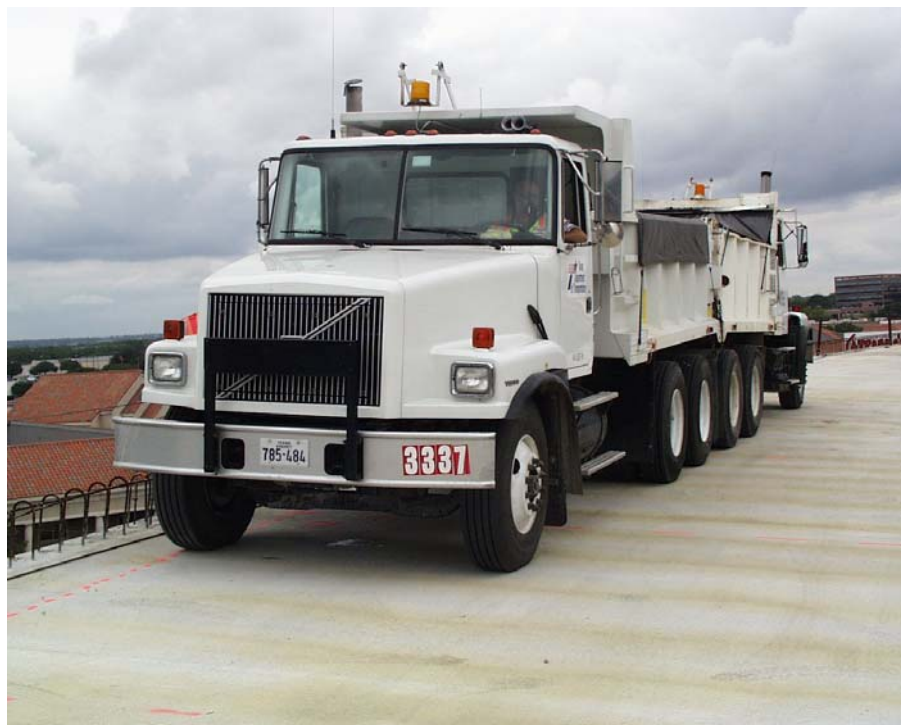
Figure 6.19 Truck Positioning During K Live Load Test
